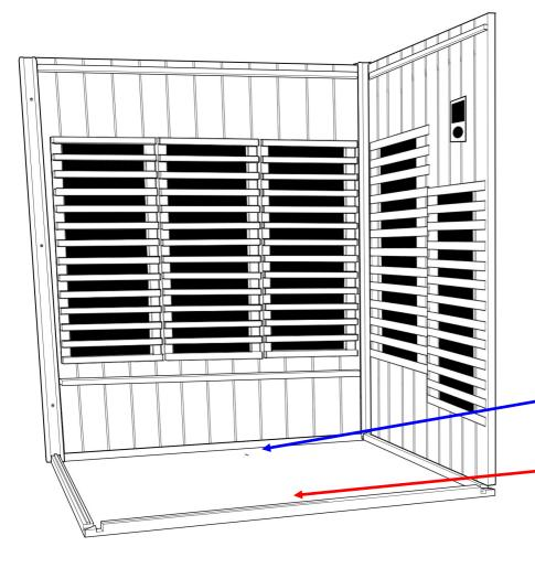
Place the front part of the floor into position next. This insert will have curved cutouts which are positioned towards the front of the sauna.
