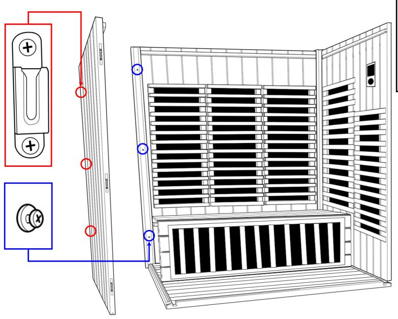
Lift the left side panel and slide the brackets up the screw fixings and lock into position. Also ensure you push the panel down onto the left bottom strut and ensure they lock together.
