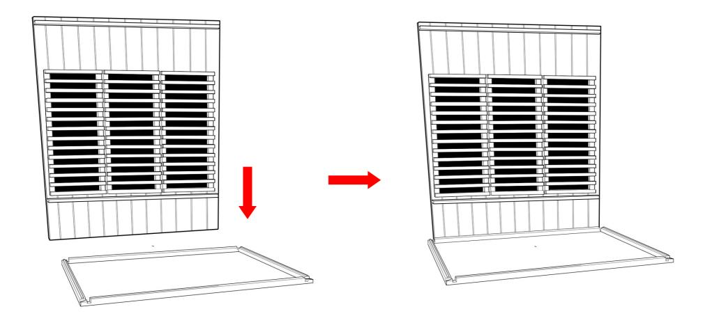
Place the back panel onto the base and slot the right post beam up to lock in position.
