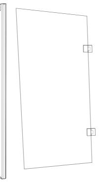
Insert the fixed glass into the groove cut-outs in the framework, lift the top framework up, then slot back down once it is in position.
