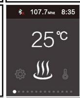
Scroll (Button 3) until you see the interface (left). Once here, press (Button 3) to enter the sauna mode. This will toggle the Sauna heater on/off as desired. Use the Time/Temp settings to make the most out of your session.
