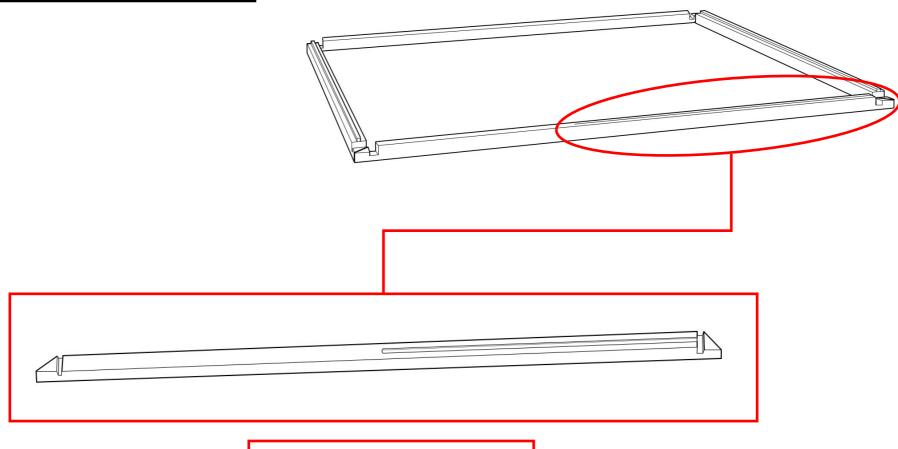
**Note:** The front strut has a groove cut out for the front fixed glass panel. Make sure this strut is at the front of the square.
