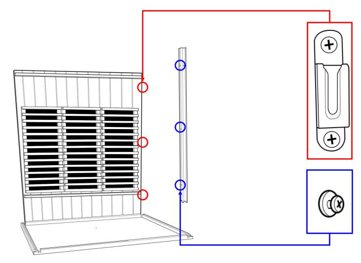
Slot the right upright post down onto the bracket to secure in place.
