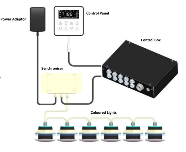
1. Connect the Power Adaptor to the Synchroniser.
