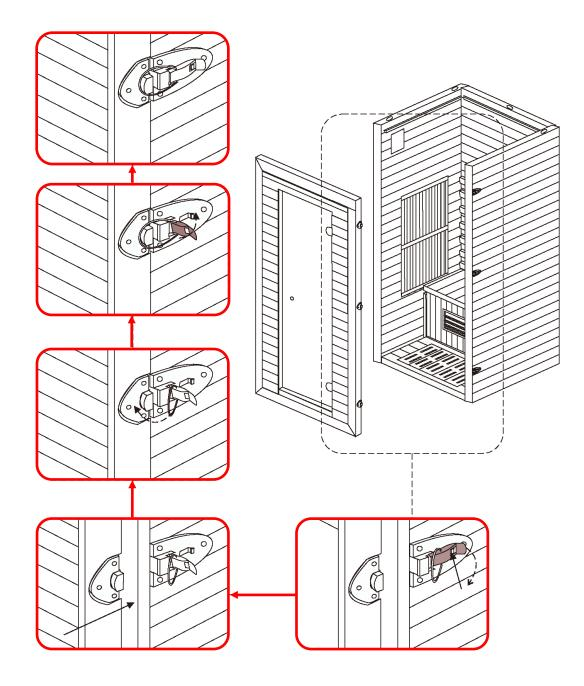
Place the door panel in line with the latches and secure with locking the latches.
