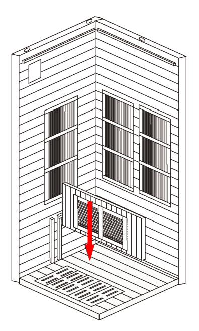
Slot the bench front panel between the grooves and fit into place.
