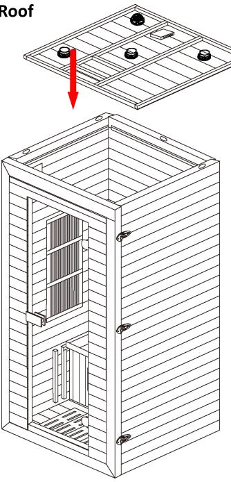
Carefully place the roof into the remaining space making sure it is resting on all sides of the fitted ledges.
