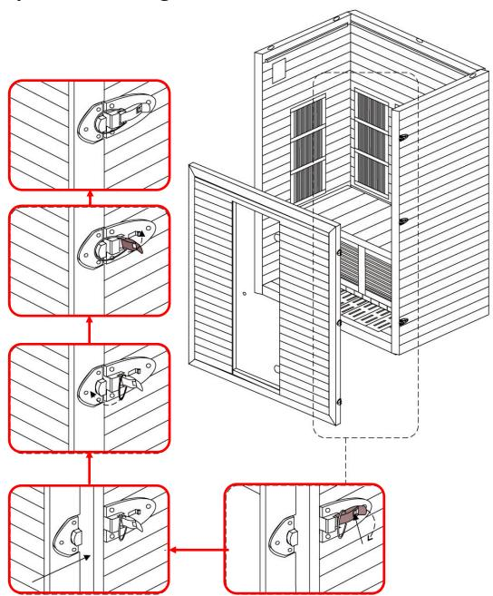
Place the door panel in line with the latches and secure with locking the latches.
