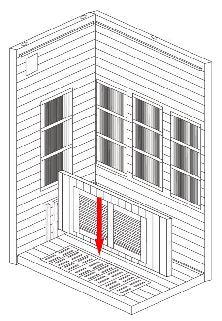
Slot the bench front panel between the grooves and fit into place.
