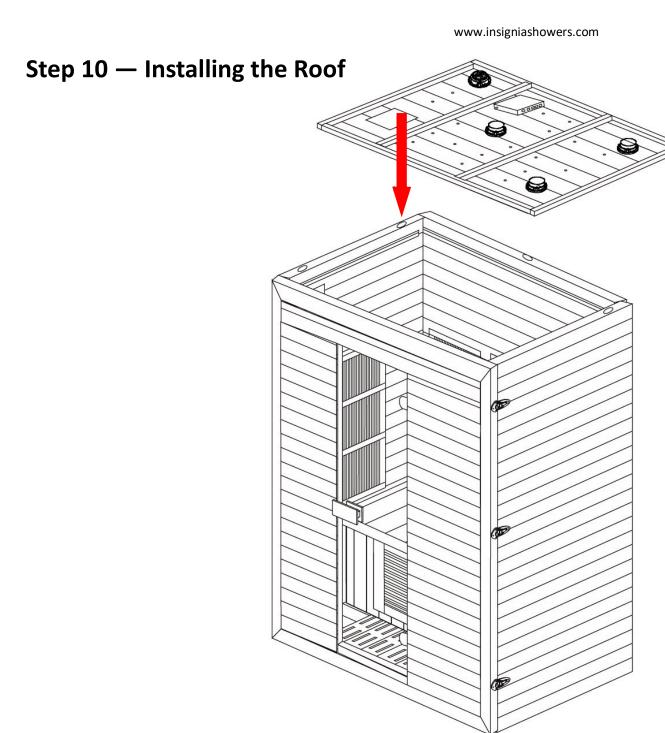
Carefully place the roof into the remaining space making sure it is resting on all sides of the fitted ledges.
