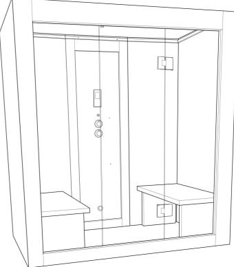
Lift the front and slot the fixing screws into the brackets on either side panel and push down to secure into position
