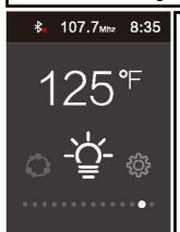
Scroll (Button 3) until you see the interface (left). Once here, press (Button 3) to turn off the 12V light. Press again to turn it on. The light will turn on automatically when the panel is turned on.
