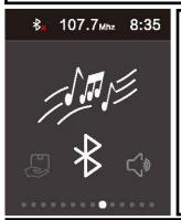
To operate the Bluetooth, scroll with (Button 3) until you see the interface (left). Scan for the control panel on your device and pair. Once paired you should hear a connection tone. Press play on your device to begin listening.
