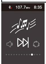
To change track whilst in the sauna form the panel, scroll to the audio interface (left). Then press the scroll (Button 3) and it will change to the next track. This will also change through the saved radio station list you have made. You can only skip forwards, not backwards.
