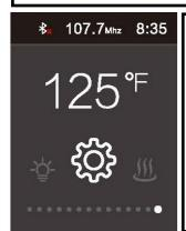
Scroll (Button 3) until you see the interface (left). Once here, press (Button 3) to enter the settings mode. Here you can set the clock which operates on a 24 hour system.
