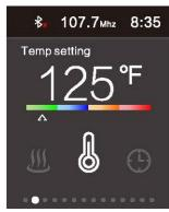
For temperature: Scroll (Button 3) until you see the interface (left). Once here, press (Button 3) to enter the temp mode.
