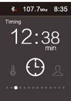
For time: Scroll (Button 3) until you see the interface (left). Once here, press (Button 3) to enter the time mode. Scroll until desired duration is set and simply press (Button 3) to confirm.
