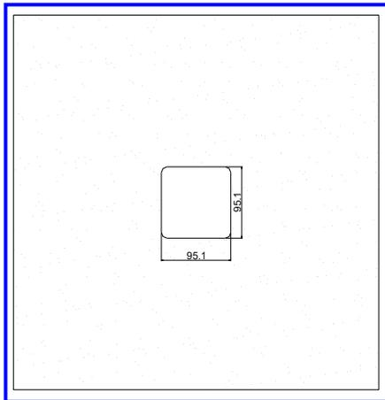
Place the housing box into the recess created.
