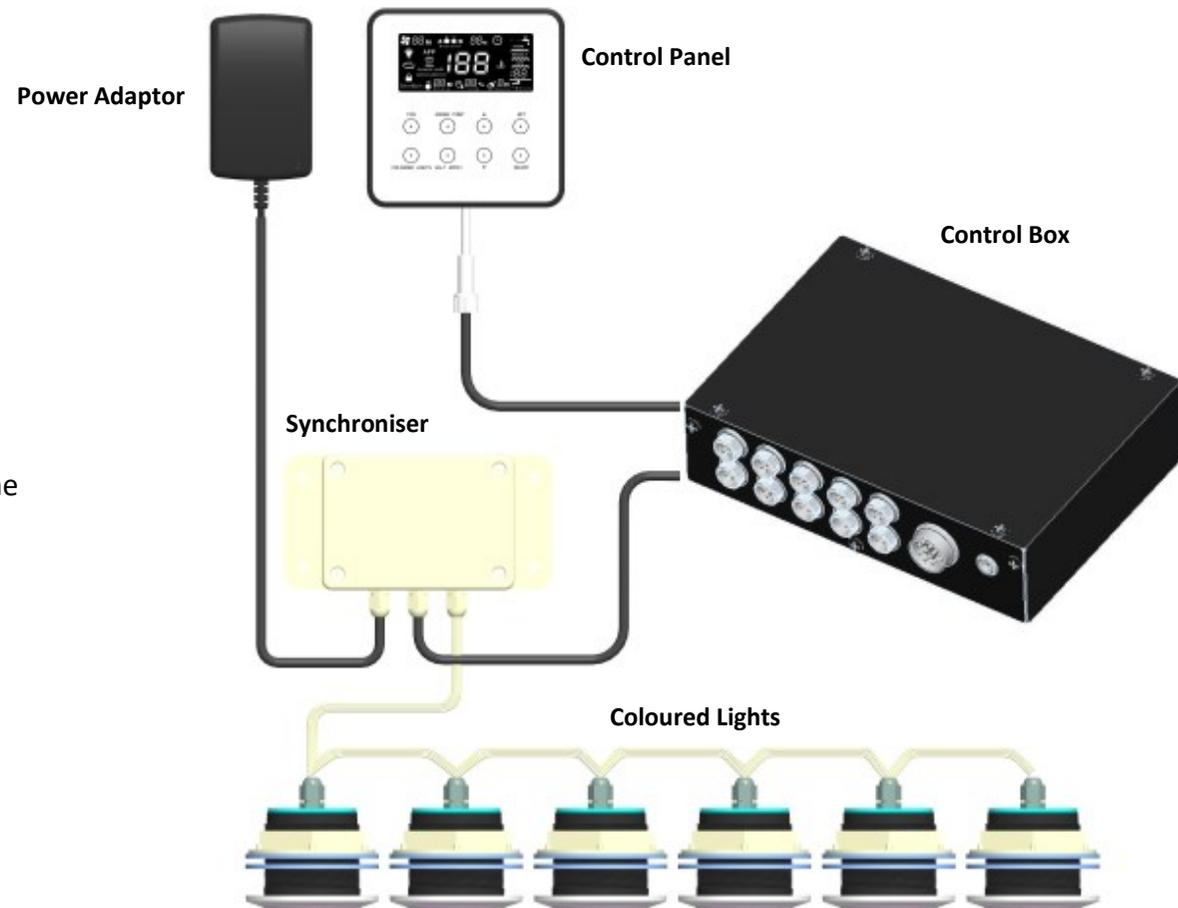
1. Connect the **Power Adaptor** to the **Synchroniser**.
