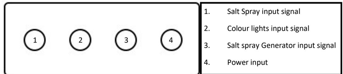
1. Connect the steam generator central box to the salt spray generator central box — DC connector 1.
