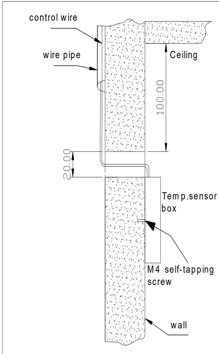
1. The control wire and temperature wire should not be parallel to the power wire.
